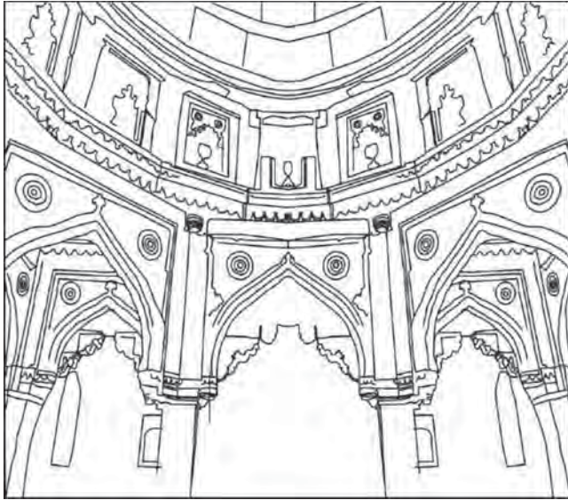
Figure 9a: Details of the squinch supporting the central dome of Chhoti Dargah
