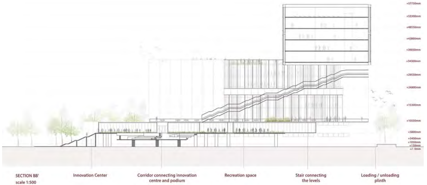
Figure 10: Section through the central podium. Source: Author, 2023
