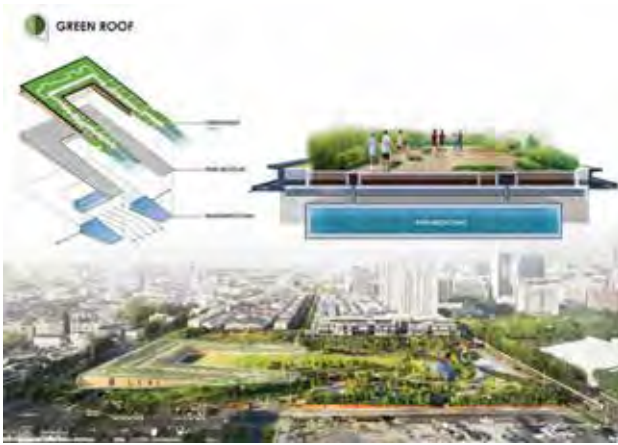
Figure 4 : View of the storage tanks and a cross section under the green roof and the museum (Source: https://time.com/collection-post/5718871/kotchakorn-voraakhom/ Accessed on 11 Dec. 2020)
