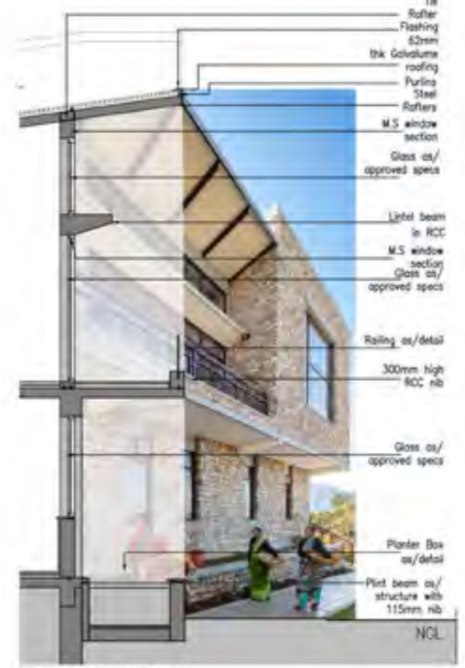
TYPICAL WALL SECTION 1:50
