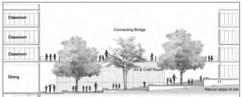
Section showing connecting bridge
