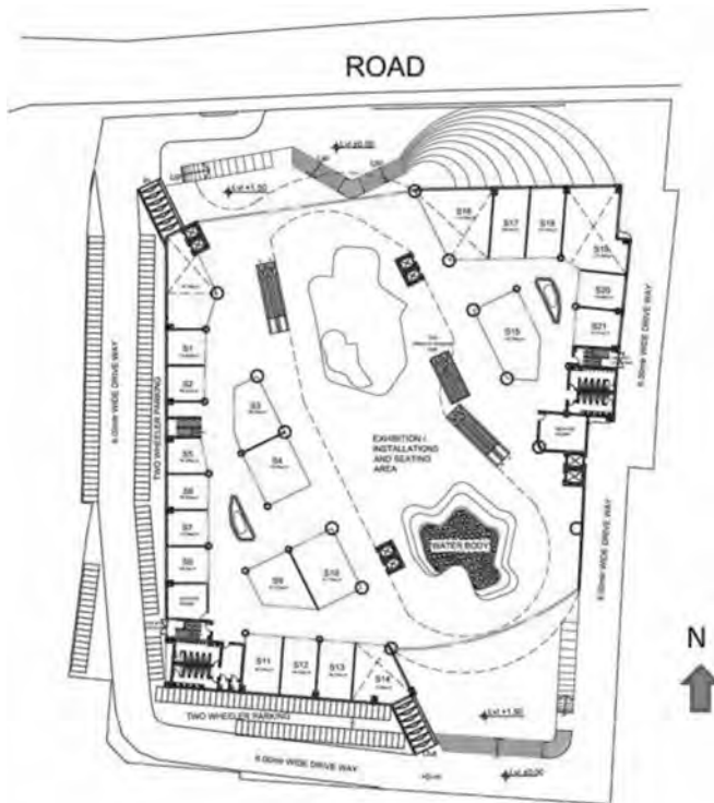
Fig. 3 : Ground, first and second floor plans showing the layout of shops. Two wheeler parking and entry-exit points to basement in ground floor.
